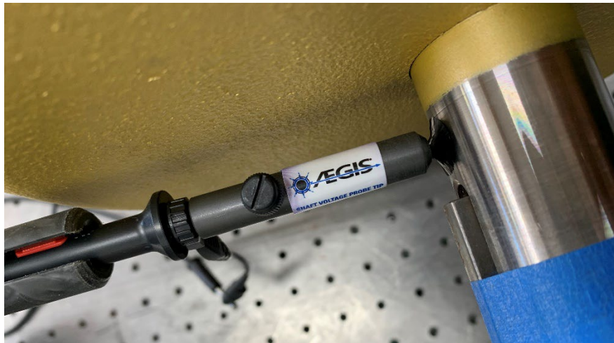
Figure 10. Induction motor test probe contact detail
