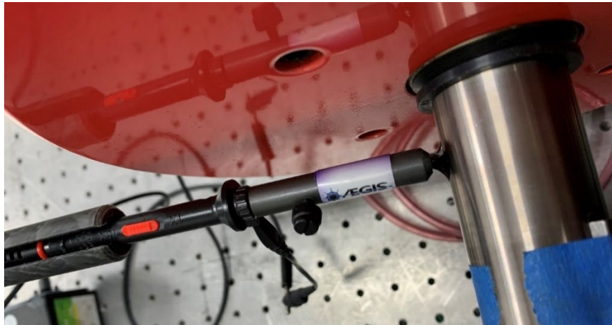
Figure 8. V03 test probe contact detail
